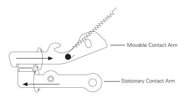
When a fault develops, current increases which increases the strength of the magnetic field. The increased strength of the opposing magnetic fields actually helps to open the contacts faster by forcing them apart.
