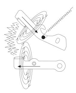
In comparison, the blow-apart contact design helps to open the contacts faster than the straight-through arrangement. I<sup>2</sup>T is greatly reduced since arc extinguishment in less than 4 milliseconds is common with blow-apart contacts. This means that electrical equipment is exposed to less heat over a shorter period of time. The result is a higher degree of protection.
