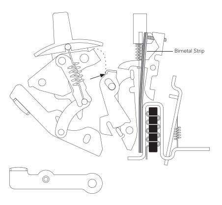
A bimetal strip is made of two dissimilar metals bonded together. The two metals have different thermal expansion characteristics, so the bimetal bends when heated. As current rises, heat also rises. The hotter the bimetal becomes the more it bends, until the mechanism is released.
