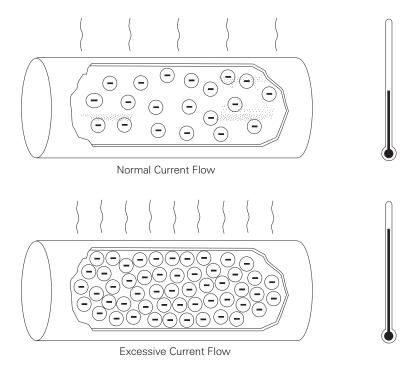
Excessive current is referred to as overcurrent. The *National Electrical Code®* (*NEC®*) defines overcurrent as *any current in excess of the rated current of equipment or the ampacity of a conductor. It may result from overload, short circuit, or ground fault* (Article 100-definitions).
