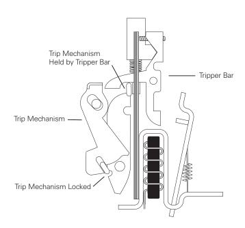
The operating mechanism is held in "ON" position by the trip mechanism. When a trip is activated, the trip mechanism releases the operating mechanism, which opens the contacts.
