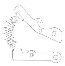
The arc can cause burning on the contacts. In addition, ionized gases form inside the molded case. If the arc isn't extinguished quickly the pressure from the ionized gases could cause the molded case to rupture. An arc chute assembly is used to quench the arc. This assembly is made up of several "U" shaped steel plates that surround the contacts. As the arc is developed it is drawn into the arc chute where it is divided into smaller arcs, which are extinguished faster.
