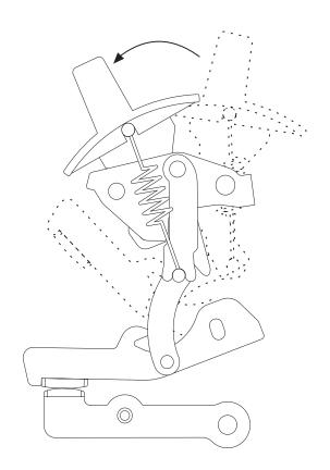
To open the contacts, the operating handle is moved from the "ON" to the "OFF" position. In this process a spring begins to apply tension to the mechanism. When the handle is directly over the center the tension in the spring is strong enough to snap the contacts open. As in closing the circuit breaker contacts, contact opening speed is independent of how fast the handle is operated.
